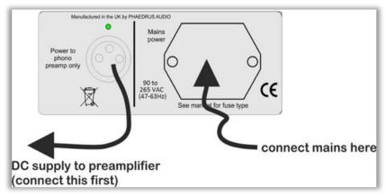
The PSU and preamplifier should be connected BEFORE mains is applied to the PSU unit. It is not dangerous or harmful to the equipment, but it is better never to
